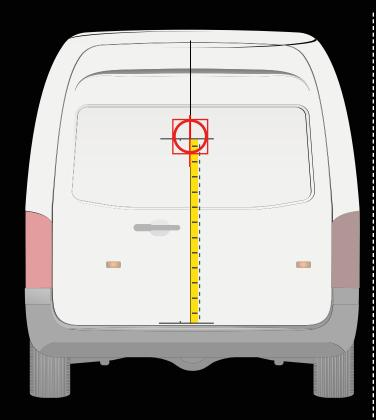
Place the drill template as shown in the picture. Place the drill temp
