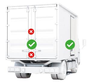
Please take into account the internal distance between the locking shafts of the doors. The drilling template indicates the minimum distances that allow installation with exposed shafts (minimum internal distance 190 mm) or recessed shafts inside the doors (minimum internal distance 150 mm). Before permanently positioning the template, check for possible interferences with external or internal elements of the doors and the vehicle's original locking systems.
